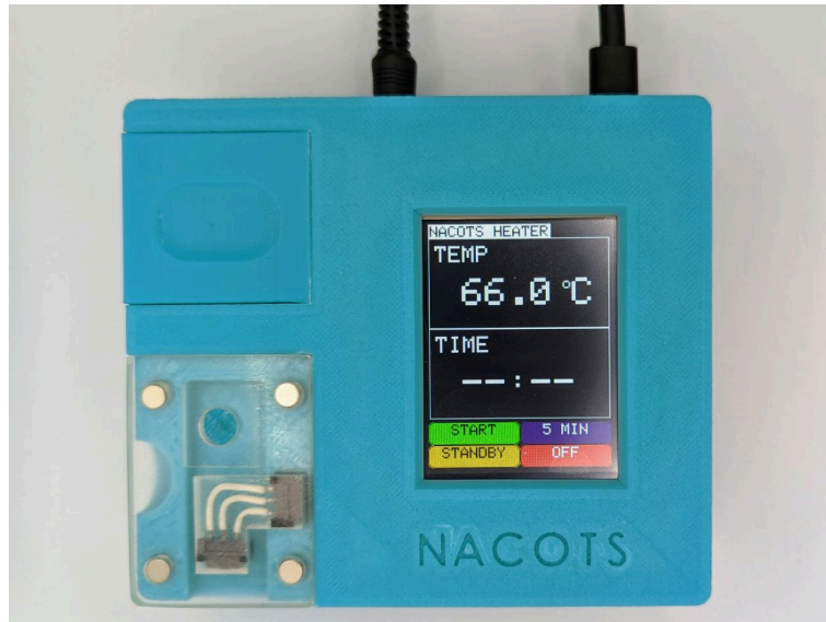
Figure 3. NACOTS device standby mode after it reaches above 65°C
