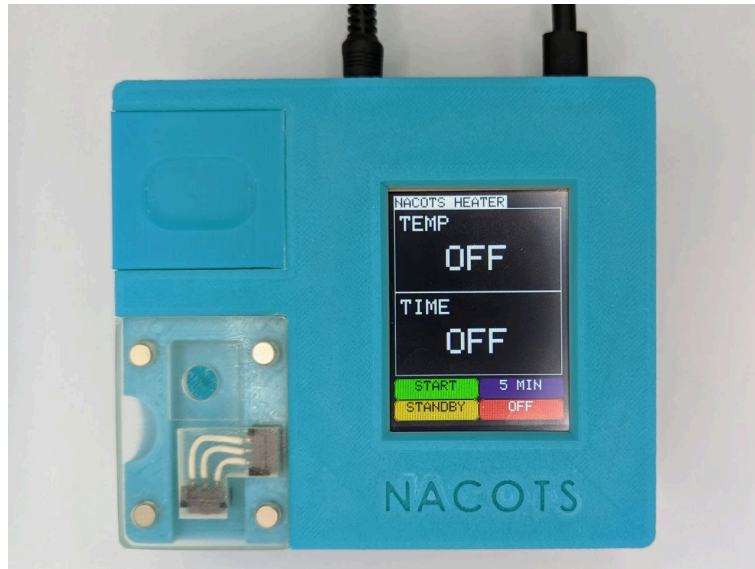
Figure 1. NACOTS device status when in idle mode
