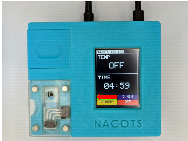
Figure 7. NACOTS device status after pressing 5 MIN button
